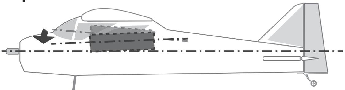
In this case, adjust so that the GYA460 is mounted slightly downward.
