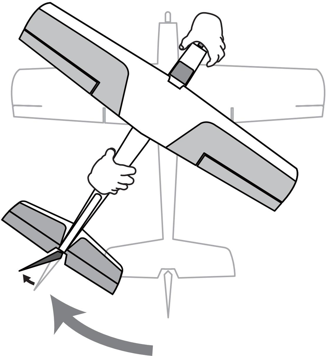
**Tilt the airplane to the left on the ground and check that the ailerons operate to the right.**
