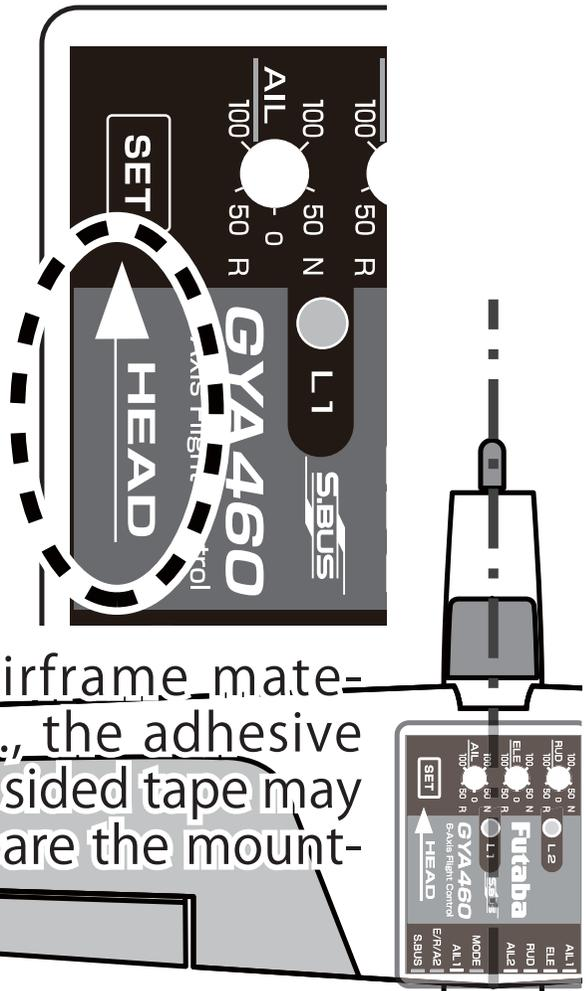
\*Depending on the airframe material such as balsa, etc., the adhesive strength of the double sided tape may drop. In this case, prepare the mounting surface well.
